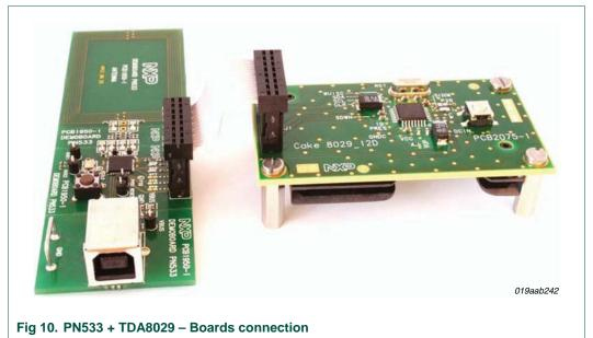
To use the board in this configuration, the connection ST1 must be closed and ST2 must be unsoldered because the PN533 uses the Energy Saving Mode of the TDA8029.
